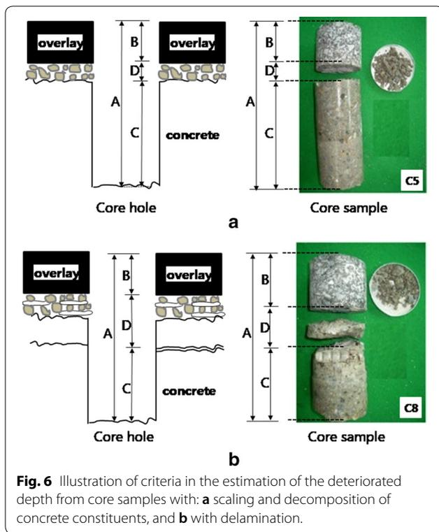
**Fig. 6** Illustration of criteria in the estimation of the deteriorated depth from core samples with: **a** scaling and decomposition of concrete constituents, and **b** with delamination.
