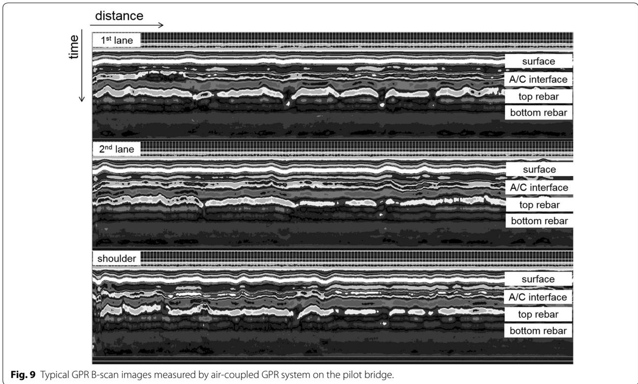
**Fig. 9** Typical GPR B-scan images measured by air-coupled GPR system on the pilot bridge.
