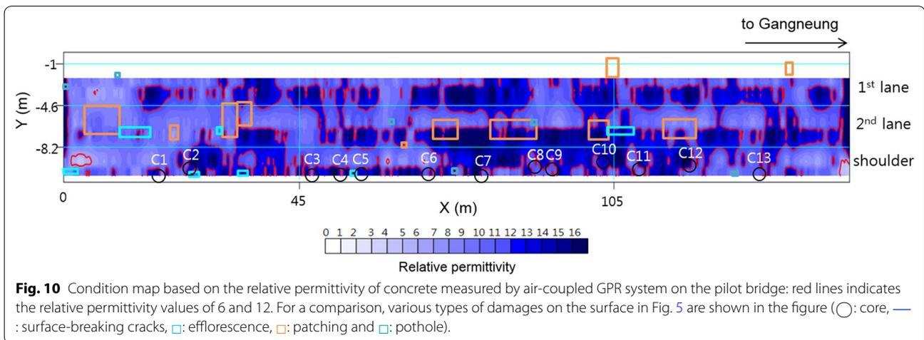
**Fig. 10** Condition map based on the relative permittivity of concrete measured by air-coupled GPR system on the pilot bridge: red lines indicates the relative permittivity values of 6 and 12. For a comparison, various types of damages on the surface in Fig. 5 are shown in the figure (○: core, —: surface-breaking cracks, □: efflorescence, □: patching and □: pothole).
