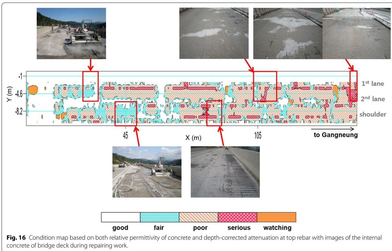
**Fig. 16** Condition map based on both relative permittivity of concrete and depth-corrected attenuation at top rebar with images of the internal concrete of bridge deck during repairing work.
