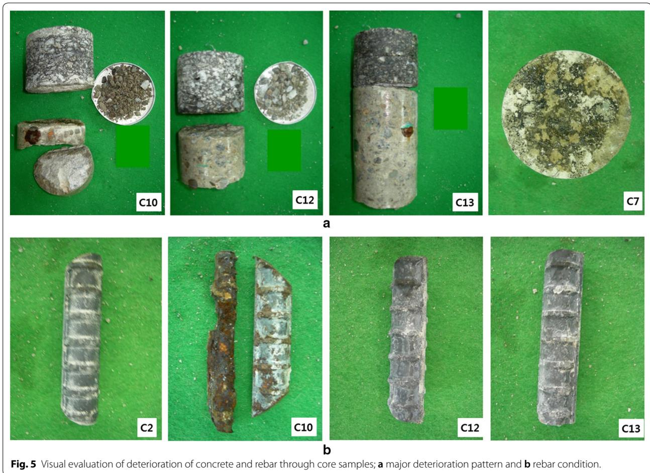
**Fig. 5** Visual evaluation of deterioration of concrete and rebar through core samples; **a** major deterioration pattern and **b** rebar condition.
