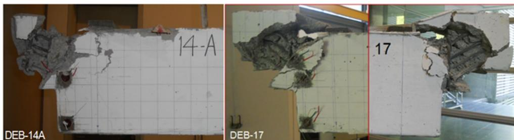
Fig. 18 The beams condition after testing (For DEB-14A and DEB-17).
