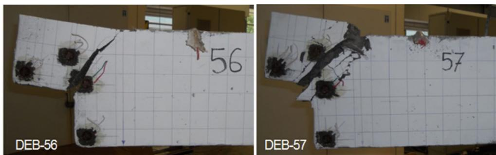
**Fig. 13** The beam condition after testing (For DEB-56 and DEB-57).
