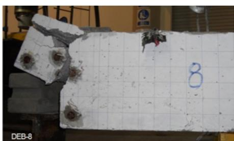
**Fig. 11** The beam condition after testing (For DEB-8).
