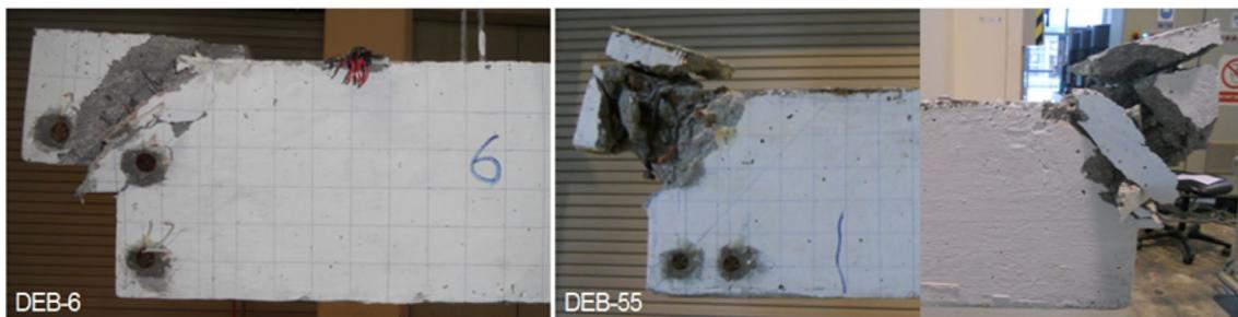
**Fig. 10** The beams condition after testing (For DEB-6 and DEB-55).
