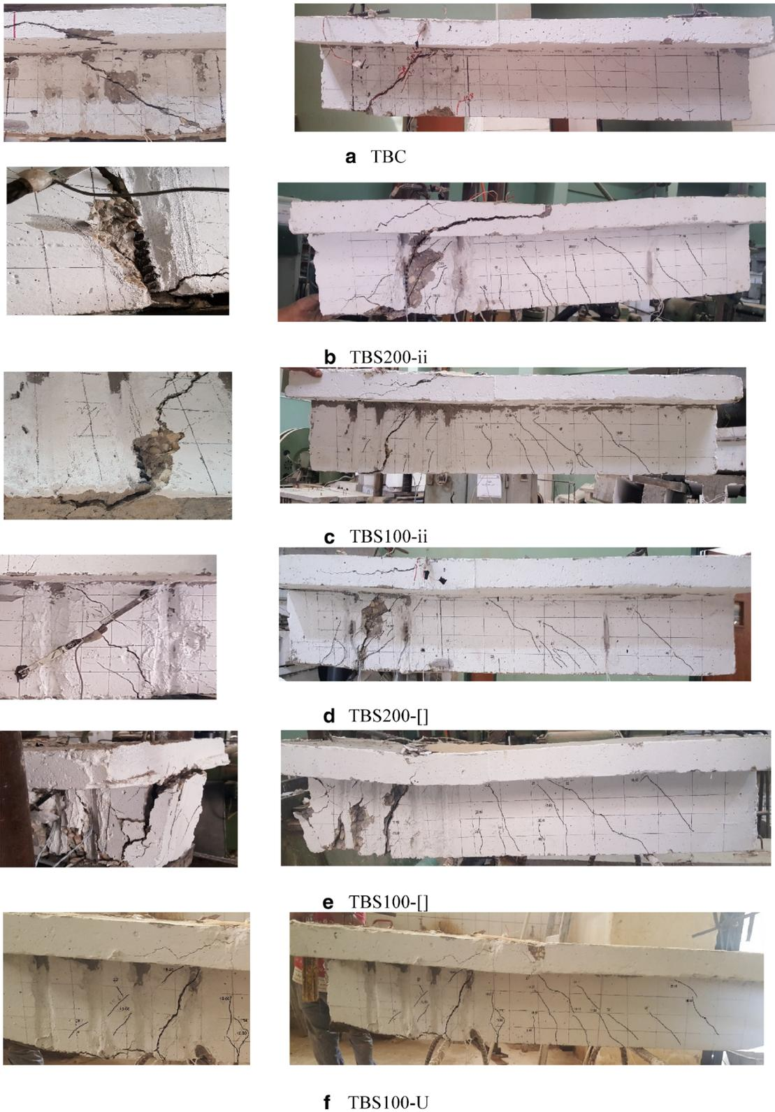
**Fig. 12** Failure modes and crack patterns of the tested beams.
