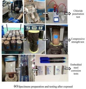
Fig. 1 Specimens preparation and testing of exposed concrete.
